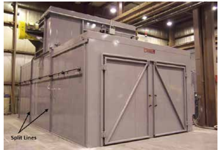
Figure 4: The body of this batch oven is designed to be split into three sections for shipment.
