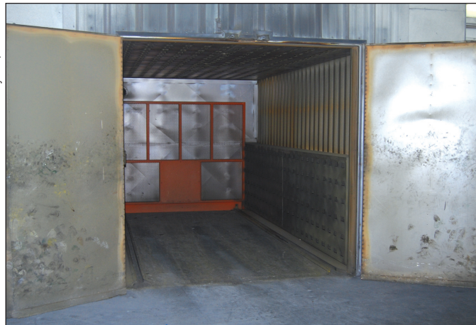
Crager's powder coats products of various sizes ranging from 2 x 3" to 12 x 7'. The 8' wide x 16' deep x 8' high work chamber of the oven provides sufficient area for the shop to process a range of sizes.
